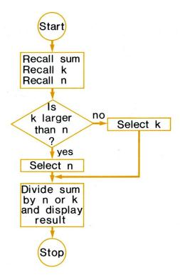
Subroutine D begins by recalling the sum from  $R_0$ , k from  $R_E$  and n from  $R_D$ . After these recalls the operational stack is as follows:
